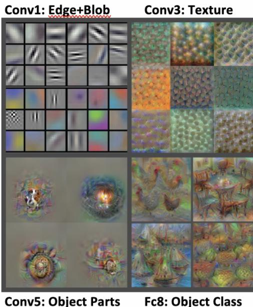
*Figure 4. Inside a convolutional network:* The figure shows representations of the AlexNet trained on the ImageNet dataset visualized by Mahendran and Vedaldi (2015).
