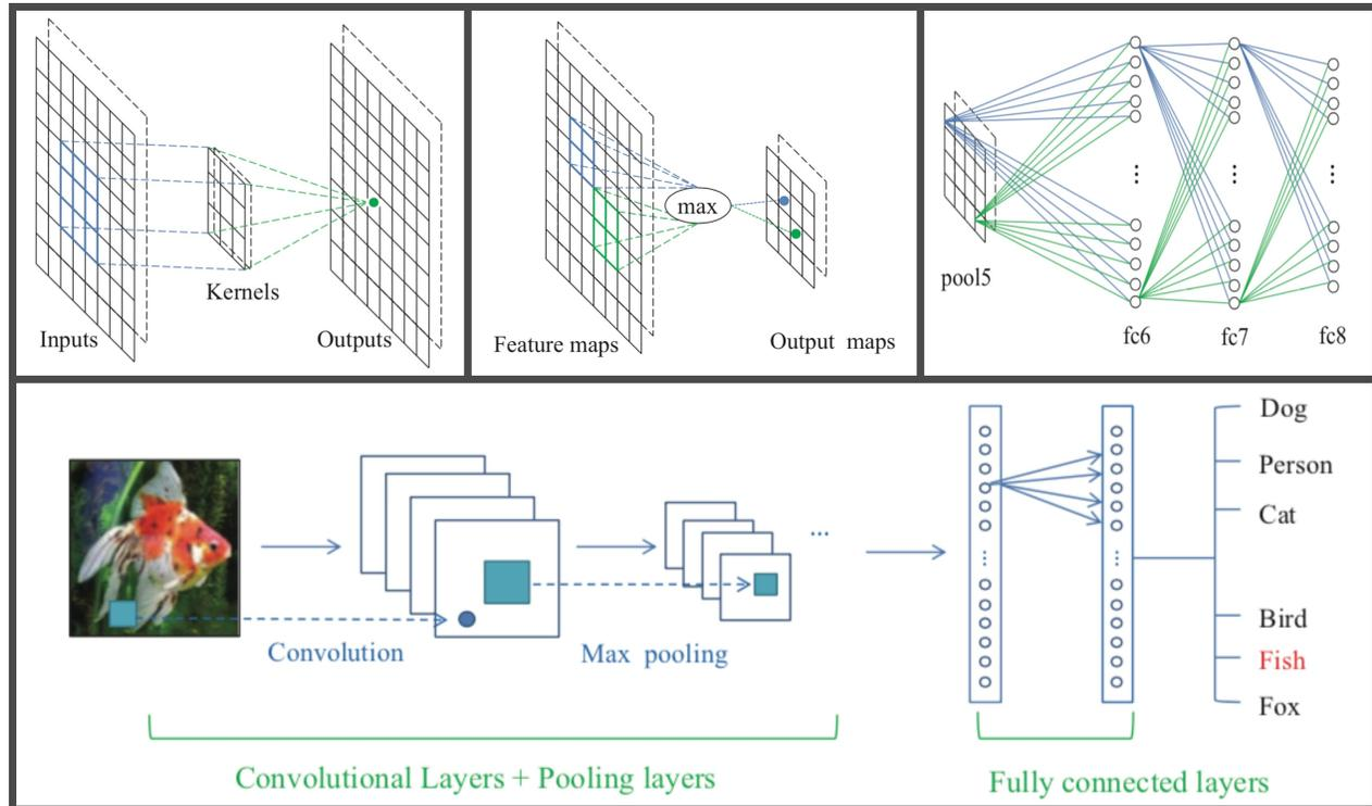
Figure 3. **Mapping mechanisms** The picture in the upper left corner shows the convolutional operation. The picture in the upper middle shows the max pooling operation and the picture on the upper right shows a schematic representation of the fully connected layers. The bottom picture summarizes the mechanisms and is a simplification of the figure 2. The pictures are taken from Yanming (2017).
